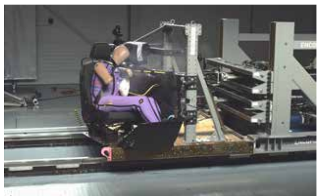
ALIS Pole Test pulse on-board (resonance-free cart without contact forces)
